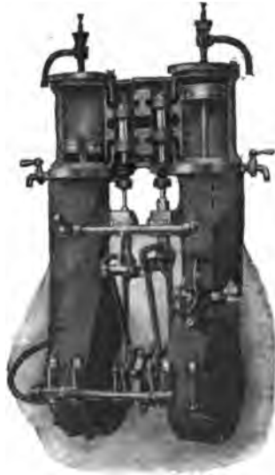
FIG. 249.—Engine of the "Toledo" Steam Carriage, showing piston valves, enclosed cranks, and relief cocks on the cylinders.
